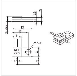
RF Solution offer a wide selection of Flanged Resistor for global customers. RFTXX-100RM1306 is a Flanged Resistor in Capacitance of 2.6 PF@100 $\Omega$ . It is made of high quality materials under a high standard, the Resistance of this product is XX  $\Omega$  (10~1500 $\Omega$  Customizable), Resistance Tolerance is  $\pm 5\%$  and Temperature Coefficient Max is 150 ppm/°C. The component has a good working performance and stability, it is ideal for handling a Power of 100 W.
