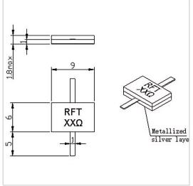
RF Solution offer a wide selection of Leaded Resistor for global customers. RFTXX-100RM0906 is a Leaded Resistor in Capacitance of 3.2 PF@100 $\Omega$ . It is made of high quality materials under a high standard, the Resistance Range of this product is XX  $\Omega$  (10-1500 $\Omega$  Customizable), Resistance Tolerance is  $\pm 5\%$  and Temperature Coefficient Max is 150 ppm/°C. The component has a good working performance and stability, it is ideal for handling a Power of 100 W.
