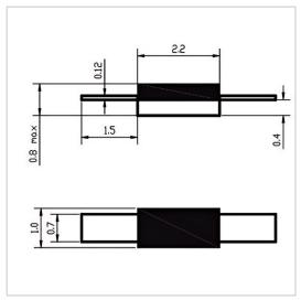
RF Solution offer a wide selection of Leaded Resistor for global customers. RFTXX-05RJ1022 is a Leaded Resistor in Resistance Range of XX  $\Omega$  (Customizable). It is made of high quality materials under a high standard, the Resistance Tolerance of this product is  $\pm 5\%$ , Substrate Material is BeO and Lead is 99.99% pure silver. The component has a good working performance and stability, it is ideal for handling a Power of 5 W.
