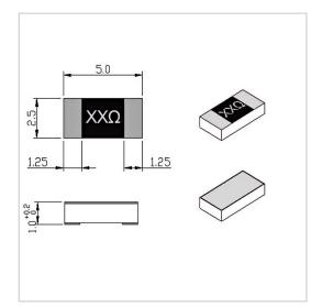
RF Solution offer a wide selection of Chip Resistor for global customers. RFTXX-05CR2550W is a Chip Resistor in Resistance Range of XX  $\Omega$  (10~3000 $\Omega$ Customizable). It is made of high quality materials under a high standard, the Resistance Tolerance of this product is ±5%, Substrate Material is BeO and Resistive Element is Thick Film. The component has a good working performance and stability, it is ideal for handling a Power of 5 W.
