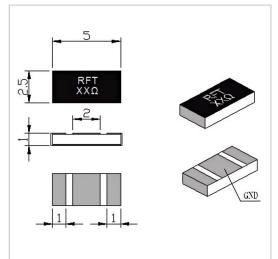
RF Solution offer a wide selection of Chip Resistor for global customers. RFTXX-05CR2550C is a Chip Resistor in Resistance Range of XX  $\Omega$  (10~3000 $\Omega$ Customizable). It is made of high quality materials under a high standard, the Resistance Tolerance of this product is ±5%, Substrate Material is BeO and Resistive Element is Thick Film. The component has a good working performance and stability, it is ideal for handling a Power of 5 W.
