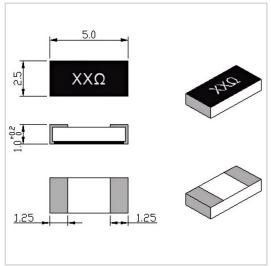
RF Solution offer a wide selection of Chip Resistor for global customers. RFTXX-05CR2550B is a Chip Resistor in Resistance Range of XX  $\Omega$  ( $10\sim3000\Omega$  Customizable). It is made of high quality materials under a high standard, the Resistance Tolerance of this product is  $\pm5\%$ , Substrate Material is BeO and Resistive Element is Thick Film. The component has a good working performance and stability, it is ideal for handling a Power of 5 W.
