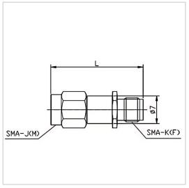
RF Solution offer a wide selection of Coaxial Fixed Attenuator for global customers. RFTXX-02RA071S-SMA-18 is a Coaxial Fixed Attenuator in Frequency Range of DC $\sim$ 18.0 GHz. It is made of high quality materials under a high standard, the VSWR Max of this product is 1.30, Attenuation Value is 0.15,20,25,30 dB and Attenuation Tolerance is 0.15,20,25,30 dB and Attenuation Tolerance and stability, it is ideal for handling a Power of 2 W.
