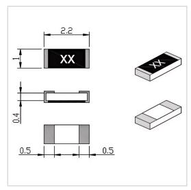
RF Solution offer a wide selection of Chip Resistor for global customers. RFTXX-02CR1022B is a Chip Resistor in Resistance Range of XX  $\Omega$  (10~3000 $\Omega$  Customizable). It is made of high quality materials under a high standard, the Resistance Tolerance of this product is  $\pm 5\%$ , Substrate Material is BeO and Resistive Element is Thick Film. The component has a good working performance and stability, it is ideal for handling a Power of 2 W.
