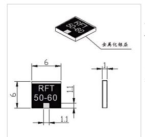
RF Solution offer a wide selection of Chip Termination for global customers. RFT50N-60WT0606 is a Chip Termination in Frequency Range of DC~6.0 GHz. It is made of high quality materials under a high standard, the Resistance Range of this product is 50  $\Omega$ , Resistance Tolerance is ±5% and VSWR Max is 1.20. The component has a good working performance and stability, it is ideal for handling a Power of 60 W.
