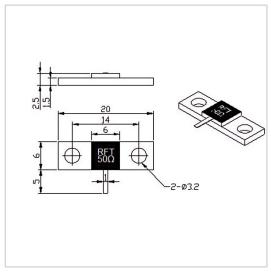
RF Solution offer a wide selection of Flanged Termination for global customers. RFT50N-60TJ2006 is a Flanged Termination in Frequency Range of DC $\sim$ 6.0 GHz. It is made of high quality materials under a high standard, the Resistance Range of this product is 50  $\Omega$ , Resistance Tolerance is  $\pm 5\%$  and VSWR Max is 1.25. The component has a good working performance and stability, it is ideal for handling a Power of 60 W.
