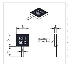
RF Solution offer a wide selection of Leaded Termination for global customers. RFT50N-60TJ0606 is a Leaded Termination in Frequency Range of DC~6.0 GHz. It is made of high quality materials under a high standard, the Resistance Range of this product is 50  $\Omega$ , Resistance Tolerance is ±5% and VSWR Max is 1.20. The component has a good working performance and stability, it is ideal for handling a Power of 60 W.
