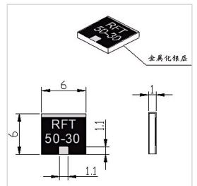
RF Solution offer a wide selection of Chip Termination for global customers. RFT50N-30WT0606 is a Chip Termination in Frequency Range of DC~6.0 GHz. It is made of high quality materials under a high standard, the Resistance Range of this product is 50  $\Omega$ , Resistance Tolerance is ±5% and VSWR Max is 1.20. The component has a good working performance and stability, it is ideal for handling a Power of 30 W.
