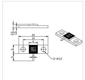
RF Solution offer a wide selection of Flanged Termination for global customers. RFT50N-30TJ2006 is a Flanged Termination in Frequency Range of DC~6.0 GHz. It is made of high quality materials under a high standard, the Resistance Range of this product is 50  $\Omega$ , Resistance Tolerance is ±5% and VSWR Max is 1.25. The component has a good working performance and stability, it is ideal for handling a Power of 30 W.
