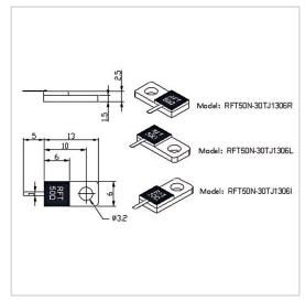
RF Solution offer a wide selection of Flanged Termination for global customers. RFT50N-30TJ1306 is a Flanged Termination in Frequency Range of DC $\sim$ 6.0 GHz. It is made of high quality materials under a high standard, the Resistance Range of this product is 50  $\Omega$ , Resistance Tolerance is  $\pm 5\%$  and VSWR Max is 1.25. The component has a good working performance and stability, it is ideal for handling a Power of 30 W.
