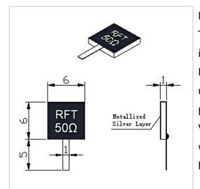
RF Solution offer a wide selection of Leaded Termination for global customers. RFT50N-30TJ0606 is a Leaded Termination in Frequency Range of DC~6.0 GHz. It is made of high quality materials under a high standard, the Resistance Range of this product is 50  $\Omega$ , Resistance Tolerance is ±5% and VSWR Max is 1.20. The component has a good working performance and stability, it is ideal for handling a Power of 30 W.
