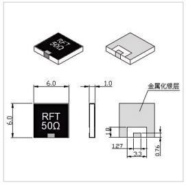
RF Solution offer a wide selection of Chip Termination for global customers. RFT50N-30CT0606 is a Chip Termination in Frequency Range of DC~6.0 GHz. It is made of high quality materials under a high standard, the Resistance Range of this product is 50  $\Omega$ , Resistance Tolerance is  $\pm 5\%$  and VSWR Max is 1.20~1.30. The component has a good working performance and stability, it is ideal for handling a Power of 30 W.
