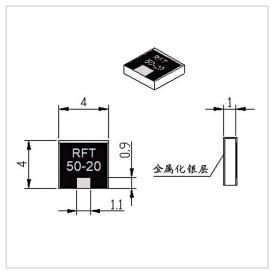
RF Solution offer a wide selection of Chip Termination for global customers. RFT50N-20WT0404 is a Chip Termination in Frequency Range of DC $\sim$ 6.0 GHz. It is made of high quality materials under a high standard, the Resistance Range of this product is 50  $\Omega$ , Resistance Tolerance is  $\pm 5\%$  and VSWR Max is  $1.20\sim1.25$ . The component has a good working performance and stability, it is ideal for handling a Power of 20 W.
