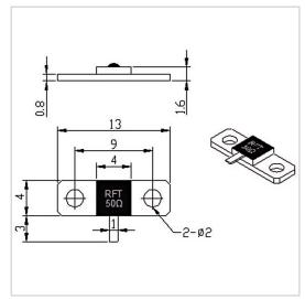
RF Solution offer a wide selection of Flanged Termination for global customers. RFT50N-20TJ1304 is a Flanged Termination in Frequency Range of DC $\sim$ 6.0 GHz. It is made of high quality materials under a high standard, the Resistance Range of this product is 50  $\Omega$ , Resistance Tolerance is  $\pm 5\%$  and VSWR Max is 1.25. The component has a good working performance and stability, it is ideal for handling a Power of 20 W.
