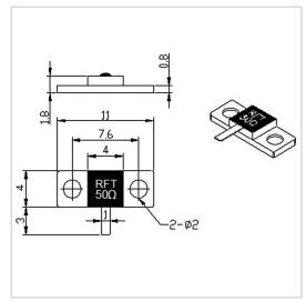
RF Solution offer a wide selection of Flanged Termination for global customers. RFT50N-20TJ1104 is a Flanged Termination in Frequency Range of DC $\sim$ 6.0 GHz. It is made of high quality materials under a high standard, the Resistance Range of this product is 50  $\Omega$ , Resistance Tolerance is  $\pm 5\%$  and VSWR Max is 1.25. The component has a good working performance and stability, it is ideal for handling a Power of 20 W.
