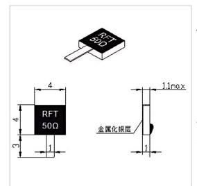
RF Solution offer a wide selection of Leaded Termination for global customers. RFT50N-20TJ0404 is a Leaded Termination in Frequency Range of DC~6.0 GHz. It is made of high quality materials under a high standard, the Resistance Range of this product is 50  $\Omega$ , Resistance Tolerance is ±5% and VSWR Max is 1.20~1.25. The component has a good working performance and stability, it is ideal for handling a Power of 20 W.
