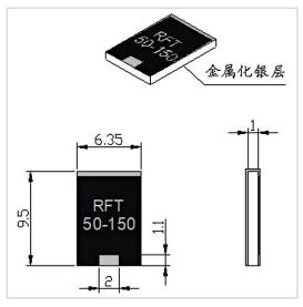
RF Solution offer a wide selection of Chip Termination for global customers. RFT50N-150WT6395 is a Chip Termination in Frequency Range of DC $\sim$ 3.0 GHz. It is made of high quality materials under a high standard, the Resistance Range of this product is 50  $\Omega$ , Resistance Tolerance is  $\pm 5\%$  and VSWR Max is 1.20. The component has a good working performance and stability, it is ideal for handling a Power of 150 W.
