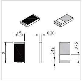
RF Solution offer a wide selection of Chip Termination for global customers. RFT50N-12CT1530 is a Chip Termination in Frequency Range of DC $\sim$ 12.0 GHz. It is made of high quality materials under a high standard, the Resistance Range of this product is 50  $\Omega$ , Resistance Tolerance is  $\pm 5\%$  and VSWR Max is 1.25. The component has a good working performance and stability, it is ideal for handling a Power of 12 W.
