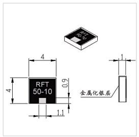
RF Solution offer a wide selection of Chip Termination for global customers. RFT50N-10WT0404 is a Chip Termination in Frequency Range of DC $\sim$ 6.0 GHz. It is made of high quality materials under a high standard, the Resistance Range of this product is 50  $\Omega$ , Resistance Tolerance is  $\pm 5\%$  and VSWR Max is  $1.20\sim1.25$ . The component has a good working performance and stability, it is ideal for handling a Power of 10 W.
