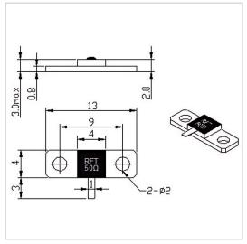
RF Solution offer a wide selection of Flanged Termination for global customers. RFT50N-10TJ1304 is a Flanged Termination in Frequency Range of DC $\sim$ 6.0 GHz. It is made of high quality materials under a high standard, the Resistance Range of this product is 50  $\Omega$ , Resistance Tolerance is  $\pm 5\%$  and VSWR Max is 1.20. The component has a good working performance and stability, it is ideal for handling a Power of 10 W.
