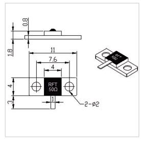
RF Solution offer a wide selection of Flanged Termination for global customers. RFT50N-10TJ1104 is a Flanged Termination in Frequency Range of DC $\sim$ 6.0 GHz. It is made of high quality materials under a high standard, the Resistance Range of this product is 50  $\Omega$ , Resistance Tolerance is  $\pm 5\%$  and VSWR Max is 1.20. The component has a good working performance and stability, it is ideal for handling a Power of 10 W.
