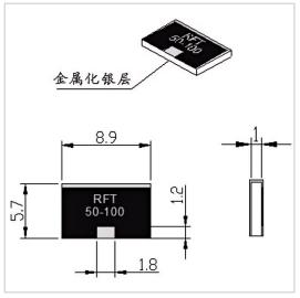
RF Solution offer a wide selection of Chip Termination for global customers. RFT50N-100WT8957 is a Chip Termination in Frequency Range of DC $\sim$ 3.0 GHz. It is made of high quality materials under a high standard, the Resistance Range of this product is 50  $\Omega$ , Resistance Tolerance is  $\pm 5\%$  and VSWR Max is 1.20. The component has a good working performance and stability, it is ideal for handling a Power of 100 W.
