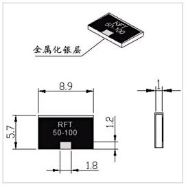
RF Solution offer a wide selection of Chip Termination for global customers. RFT50N-100WT8957B is a Chip Termination in Frequency Range of DC $\sim$ 6.0 GHz. It is made of high quality materials under a high standard, the Resistance Range of this product is 50  $\Omega$ , Resistance Tolerance is  $\pm 5\%$  and VSWR Max is 1.25. The component has a good working performance and stability, it is ideal for handling a Power of 100 W.
