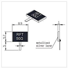
RF Solution offer a wide selection of Leaded Termination for global customers. RFT50N-100TJ8957 is a Leaded Termination in Frequency Range of DC $\sim$ 3.0 GHz. It is made of high quality materials under a high standard, the Resistance Range of this product is 50  $\Omega$ , Resistance Tolerance is  $\pm 5\%$  and VSWR Max is 1.20. The component has a good working performance and stability, it is ideal for handling a Power of 100 W.
