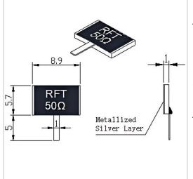
RF Solution offer a wide selection of Leaded Termination for global customers. RFT50N-100TJ8957B is a Leaded Termination in Frequency Range of DC~6.0 GHz. It is made of high quality materials under a high standard, the Resistance Range of this product is 50  $\Omega$ , Resistance Tolerance is ±5% and VSWR Max is 1.20. The component has a good working performance and stability, it is ideal for handling a Power of 100 W.
