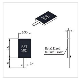
RF Solution offer a wide selection of Leaded Termination for global customers. RFT50N-100TJ6395 is a Leaded Termination in Frequency Range of DC $\sim$ 3.0 GHz. It is made of high quality materials under a high standard, the Resistance Range of this product is 50  $\Omega$ , Resistance Tolerance is  $\pm 5\%$  and VSWR Max is 1.20. The component has a good working performance and stability, it is ideal for handling a Power of 100 W.
