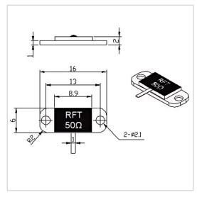
RF Solution offer a wide selection of Flanged Termination for global customers. RFT50N-100TJ1606B is a Flanged Termination in Frequency Range of DC $\sim$ 6.0 GHz. It is made of high quality materials under a high standard, the Resistance Range of this product is 50  $\Omega$ , Resistance Tolerance is  $\pm 5\%$  and VSWR Max is 1.20. The component has a good working performance and stability, it is ideal for handling a Power of 100 W.
