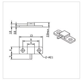
RF Solution offer a wide selection of Flanged Termination for global customers. RFT50A-10TM1304 is a Flanged Termination in Frequency Range of DC $\sim$ 6.0 GHz. It is made of high quality materials under a high standard, the Resistance Range of this product is 50  $\Omega$ , Resistance Tolerance is  $\pm 5\%$  and VSWR Max is 1.20. The component has a good working performance and stability, it is ideal for handling a Power of 10 W.
