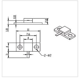
RF Solution offer a wide selection of Flanged Termination for global customers. RFT50A-10TM1104 is a Flanged Termination in Frequency Range of DC $\sim$ 6.0 GHz. It is made of high quality materials under a high standard, the Resistance Range of this product is 50  $\Omega$ , Resistance Tolerance is  $\pm 5\%$  and VSWR Max is 1.20. The component has a good working performance and stability, it is ideal for handling a Power of 10 W.
