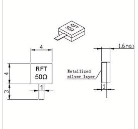
RF Solution offer a wide selection of Leaded Termination for global customers. RFT50A-10TM0404 is a Leaded Termination in Frequency Range of DC~6.0 GHz. It is made of high quality materials under a high standard, the Resistance Range of this product is 50  $\Omega$ , Resistance Tolerance is ±5% and VSWR Max is 1.20. The component has a good working performance and stability, it is ideal for handling a Power of 10 W.
