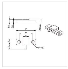
RF Solution offer a wide selection of Flanged Termination for global customers. RFT50A-05TM1304 is a Flanged Termination in Frequency Range of DC $\sim$ 6.0 GHz. It is made of high quality materials under a high standard, the Resistance Range of this product is 50  $\Omega$ , Resistance Tolerance is  $\pm 5\%$  and VSWR Max is 1.20. The component has a good working performance and stability, it is ideal for handling a Power of 5 W.
