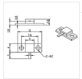
RF Solution offer a wide selection of Flanged Termination for global customers. RFT50A-05TM1104 is a Flanged Termination in Frequency Range of DC~6.0 GHz. It is made of high quality materials under a high standard, the Resistance Range of this product is 50  $\Omega$ , Resistance Tolerance is ±5% and VSWR Max is 1.20. The component has a good working performance and stability, it is ideal for handling a Power of 5 W.
