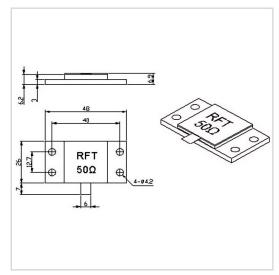
RF Solution offer a wide selection of Flanged Termination for global customers. RFT50-800TM4826 is a Flanged Termination in Frequency Range of DC $\sim$ 1.0 GHz. It is made of high quality materials under a high standard, the Resistance Range of this product is 50  $\Omega$ , Resistance Tolerance is  $\pm 5\%$  and VSWR Max is 1.20. The component has a good working performance and stability, it is ideal for handling a Power of 800 W.
