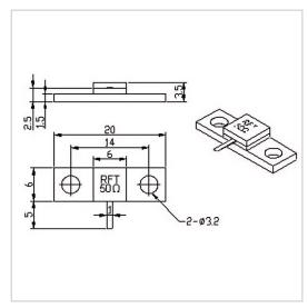
RF Solution offer a wide selection of Flanged Termination for global customers. RFT50-60TM2006 is a Flanged Termination in Frequency Range of DC $\sim$ 6.0 GHz. It is made of high quality materials under a high standard, the Resistance Range of this product is 50  $\Omega$ , Resistance Tolerance is  $\pm 5\%$  and VSWR Max is 1.25. The component has a good working performance and stability, it is ideal for handling a Power of 60 W.
