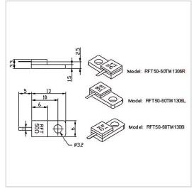
RF Solution offer a wide selection of Flanged Termination for global customers. RFT50-60TM1306 is a Flanged Termination in Frequency Range of DC $\sim$ 6.0 GHz. It is made of high quality materials under a high standard, the Resistance Range of this product is 50  $\Omega$ , Resistance Tolerance is  $\pm 5\%$  and VSWR Max is 1.25. The component has a good working performance and stability, it is ideal for handling a Power of 60 W.
