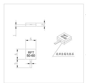
RF Solution offer a wide selection of Leaded Termination for global customers. RFT50-60TM0606 is a Leaded Termination in Frequency Range of DC~6.0 GHz. It is made of high quality materials under a high standard, the Resistance Range of this product is 50  $\Omega$ , Resistance Tolerance is ±5% and VSWR Max is 1.25. The component has a good working performance and stability, it is ideal for handling a Power of 60 W.
