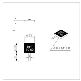
RF Solution offer a wide selection of Leaded Termination for global customers. RFT50-60TJ6363 is a Leaded Termination in Frequency Range of DC $\sim$ 6.0 GHz. It is made of high quality materials under a high standard, the Resistance Range of this product is 50  $\Omega$ , Resistance Tolerance is  $\pm 5\%$  and VSWR Max is 1.25. The component has a good working performance and stability, it is ideal for handling a Power of 60 W.
