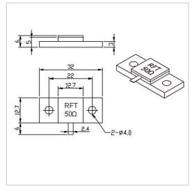
RF Solution offer a wide selection of Flanged Termination for global customers. RFT50-500TM3213 is a Flanged Termination in Frequency Range of DC~2.0 GHz. It is made of high quality materials under a high standard, the Resistance Range of this product is 50  $\Omega$ , Resistance Tolerance is  $\pm 5\%$  and VSWR Max is 1.20. The component has a good working performance and stability, it is ideal for handling a Power of 300 W.
