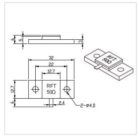
RF Solution offer a wide selection of Flanged Termination for global customers. RFT50-400TM3213 is a Flanged Termination in Frequency Range of DC~2.0 GHz. It is made of high quality materials under a high standard, the Resistance Range of this product is 50  $\Omega$ , Resistance Tolerance is  $\pm 5\%$  and VSWR Max is 1.20. The component has a good working performance and stability, it is ideal for handling a Power of 300 W.
