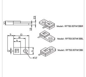
RF Solution offer a wide selection of Flanged Termination for global customers. RFT50-30TM1306 is a Flanged Termination in Frequency Range of DC~6.0 GHz. It is made of high quality materials under a high standard, the Resistance Range of this product is 50  $\Omega$ , Resistance Tolerance is ±5% and VSWR Max is 1.25. The component has a good working performance and stability, it is ideal for handling a Power of 30 W.
