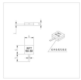
RF Solution offer a wide selection of Leaded Termination for global customers. RFT50-30TM0606 is a Leaded Termination in Frequency Range of DC $\sim$ 6.0 GHz. It is made of high quality materials under a high standard, the Resistance Range of this product is 50  $\Omega$ , Resistance Tolerance is  $\pm 5\%$  and VSWR Max is 1.25. The component has a good working performance and stability, it is ideal for handling a Power of 30 W.
