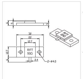
RF Solution offer a wide selection of Flanged Termination for global customers. RFT50-300TM3213B is a Flanged Termination in Frequency Range of DC~3.0 GHz. It is made of high quality materials under a high standard, the Resistance Range of this product is 50  $\Omega$ , Resistance Tolerance is ±5% and VSWR Max is 1.20~1.30. The component has a good working performance and stability, it is ideal for handling a Power of 300 W.
