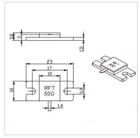
RF Solution offer a wide selection of Flanged Termination for global customers. RFT50-300TM2310 is a Flanged Termination in Frequency Range of DC $\sim$ 3.0 GHz. It is made of high quality materials under a high standard, the Resistance Range of this product is 50  $\Omega$ , Resistance Tolerance is  $\pm 5\%$  and VSWR Max is 1.20. The component has a good working performance and stability, it is ideal for handling a Power of 300 W.
