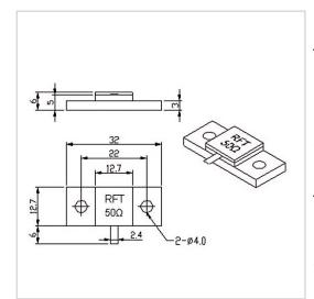
RF Solution offer a wide selection of Flanged Termination for global customers. RFT50-250TM3213B is a Flanged Termination in Frequency Range of DC~10.0 GHz. It is made of high quality materials under a high standard, the Resistance Range of this product is 50  $\Omega$ , Resistance Tolerance is ±5% and VSWR Max is 1.20~1.30. The component has a good working performance and stability, it is ideal for handling a Power of 250 W.
