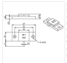
RF Solution offer a wide selection of Flanged Termination for global customers. RFT50-250TM2710 is a Flanged Termination in Frequency Range of DC~3.0 GHz. It is made of high quality materials under a high standard, the Resistance Range of this product is 50  $\Omega$ , Resistance Tolerance is ±5% and VSWR Max is 1.20. The component has a good working performance and stability, it is ideal for handling a Power of 250 W.
