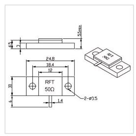
RF Solution offer a wide selection of Flanged Termination for global customers. RFT50-250TM2510 is a Flanged Termination in Frequency Range of DC $\sim$ 3.0 GHz. It is made of high quality materials under a high standard, the Resistance Range of this product is 50  $\Omega$ , Resistance Tolerance is  $\pm 5\%$  and VSWR Max is 1.20. The component has a good working performance and stability, it is ideal for handling a Power of 250 W.
